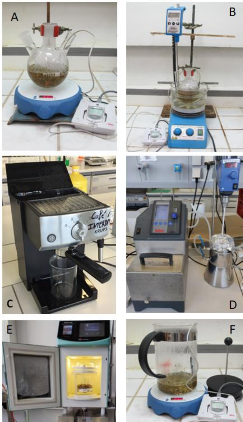
Figure S2. Picture of the experimental set-up used for each extraction mode (A: infusion; B: maceration; C: percolation; D: ultrasonic; E: Microwave; F: infusion using a French-Press Bodum® (with or without stirring)).
