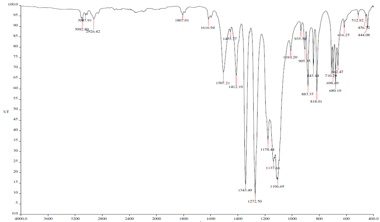
Figure S41. ATR-FTIR Spectra of Pb(SC_6H_3(CF_3)_2-3,5)_2
