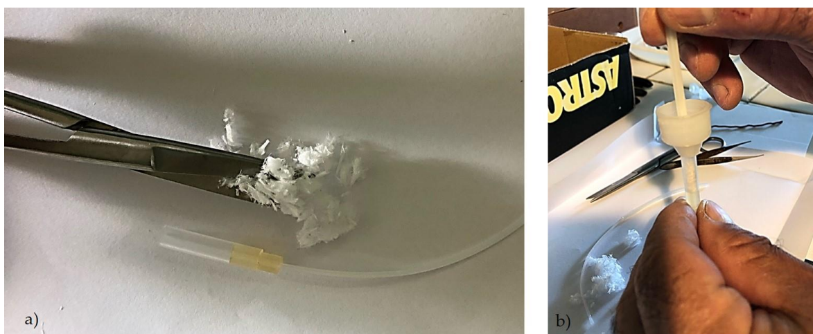
Figure S1. Preparation of the microcolumn packed with sol-gel PDPS coated glass fiber: a) cutting of glass fibers; b) packing with GF coated with sol-gel PDPS.
