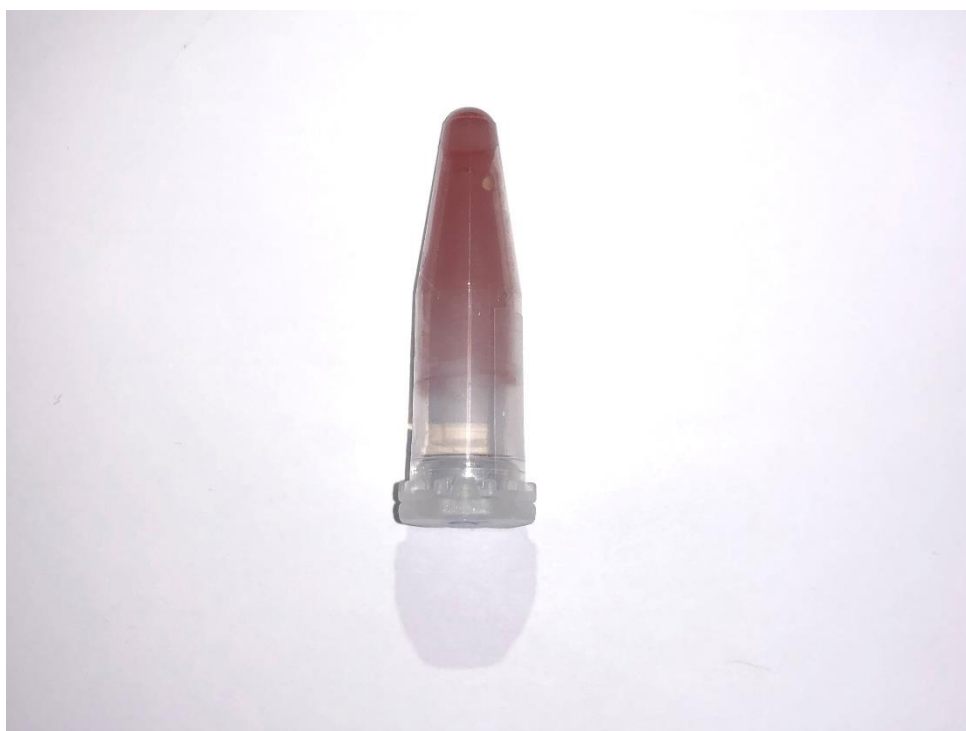
Figure S 17. Red selenium precipitate formed during catalysis of SEA/MPA exchange in the presence of catalyst 14 (200 mM).
