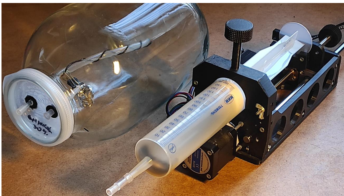
Figure S64. Vapor vessels, the 3 L glass vessel on the left, and the 160 mL syringe vessel installed onto the syringe driver on the right.
