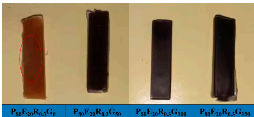
Figure S5. Pictures for anti-electrostatic test of P_{80}E_{20}R_{0.3}G_0 , P_{80}E_{20}R_{0.3}G_{50} , P_{80}E_{20}R_{0.3}G_{100} and P_{80}E_{20}R_{0.3}G_{150} samples stored after one week in the ambient environment
