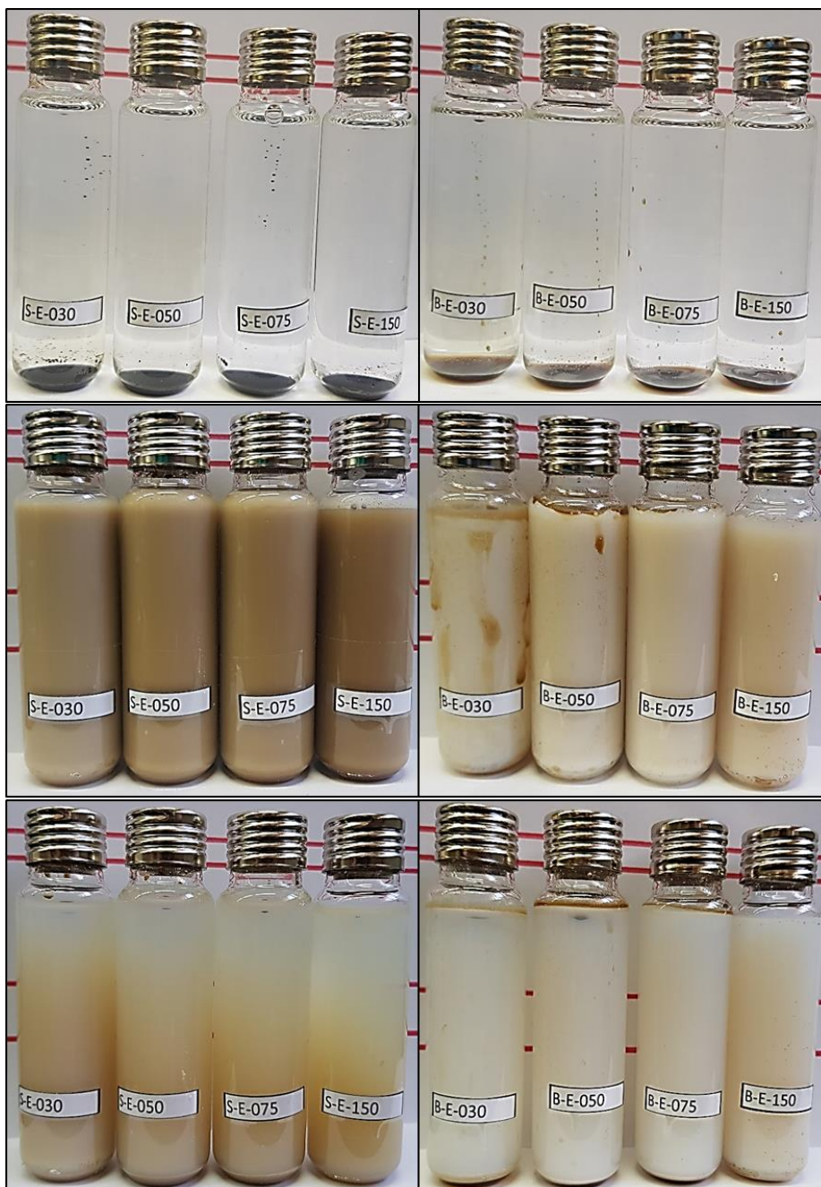
Figure S1. Left: organic phase S; Right: organic phase B adding E3 at several concentrations (Initial surfactant concentration from the left to the right: 3, 5, 7.5 and 15 g L -1 ) and pH=7. Top: Appearance before agitation. Centrum: Appearance after agitation (5h). Bottom: Appearance after 75 h of settling.
