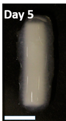
Figure S1. Uniaxial strip after being in an oxidative media for 5 days.
