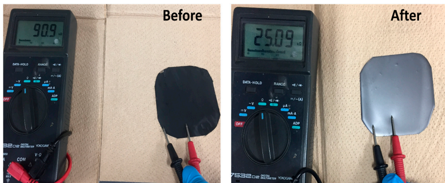
Figure S1. Photos of resistance measurement of the graphene layer before and after smoothing wiping.
