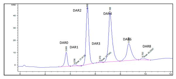
**Supplemental Figure 1.** The average drug to antibody ratios (DAR) were calculated from the integrated areas of the DAR species resolved by hydrophobic interaction chromatography detected at UV 280 nm. (A) Unlabeled reference polatuzumab vedotin with a DAR ~3.4. (B) [<sup>3</sup>H]-MMAE-polatuzumab vedotin with a DAR ~3.4.
