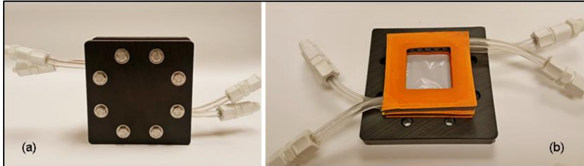
Figure S3. The 25 cm 2 pervaporation cell assembled outside view shown in (a). The pervaporation cell internal view is shown in (b), showing one of the membranes (Targray) being positioned in the cell for testing.
